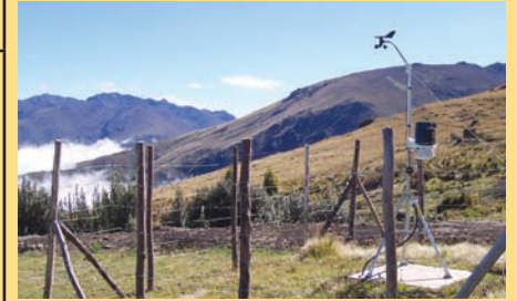
High in the mountains of Ecuador, Ed Bohn of the International Minerals Corp. uses a Vantage Pro to record baseline meteorological data for their gold exploration program.
